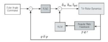
Once the longitudinal ( $\delta$ -long), lateral ( $\delta$ -lat), and yaw ( $\delta$ -yaw) are read the controller can interpret them into angular velocities of the rotors and the angle of attack necessary the UAV needs in yaw this is shown in Figure 91.
