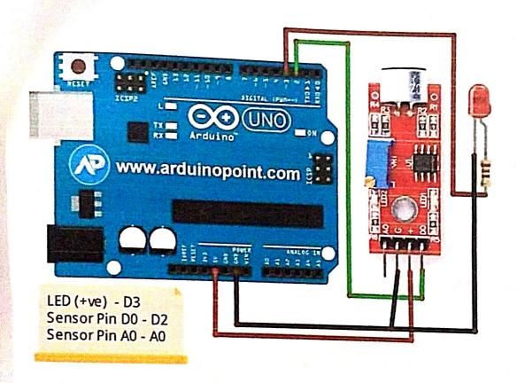
Resistor's one terminal goes to LED and another terminal goes to digital pin 3.
