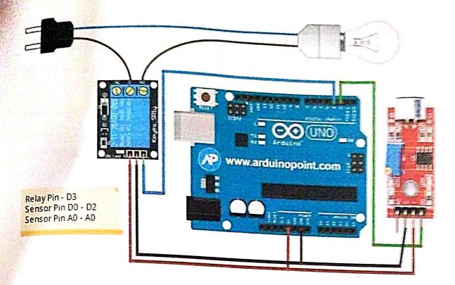
A bulb connects with a 5V relay module's NO pin and NC pin.
